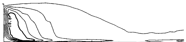
Fig. 7 NO mass fraction distribution X1000 for the combustion of H_2 with air, v_{inj} = 0.05 m/s.
